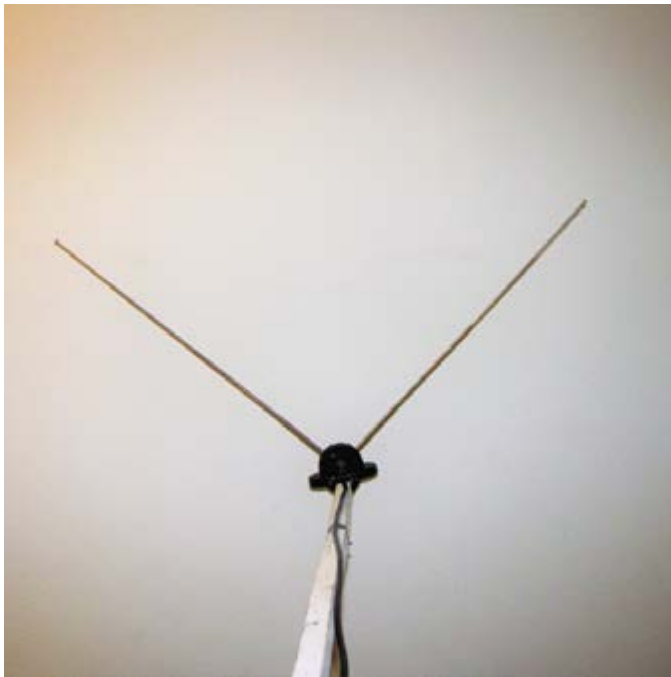
Figure 4. 2M vee dipole
