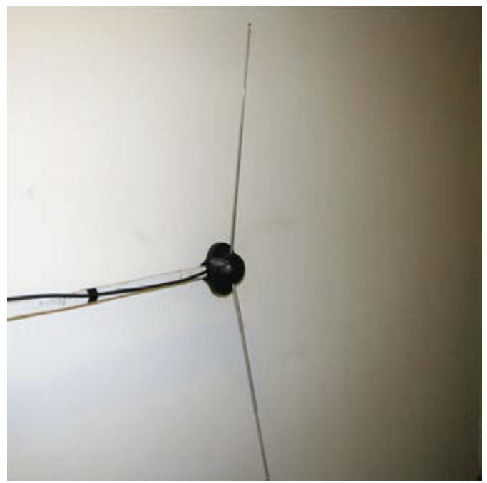
Figure 5. 2M vertical dipole.
