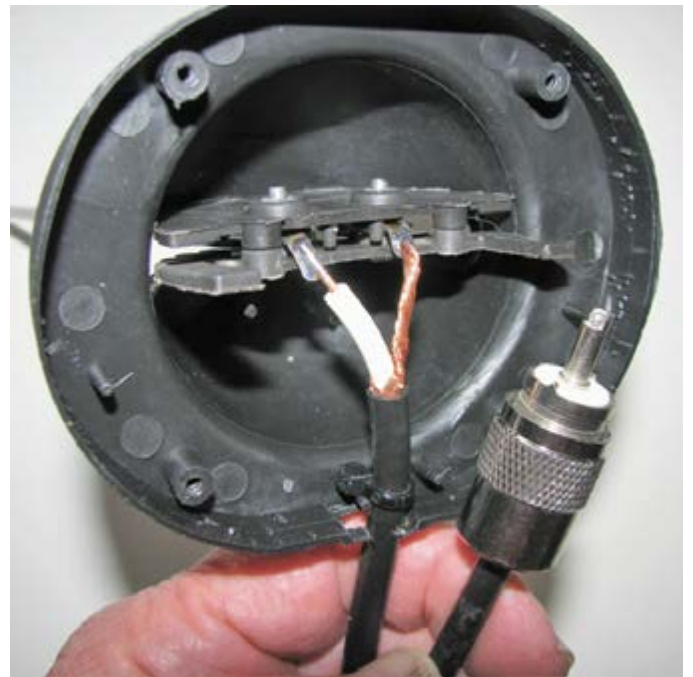
Figure 3. 50-ohm cable, new.
